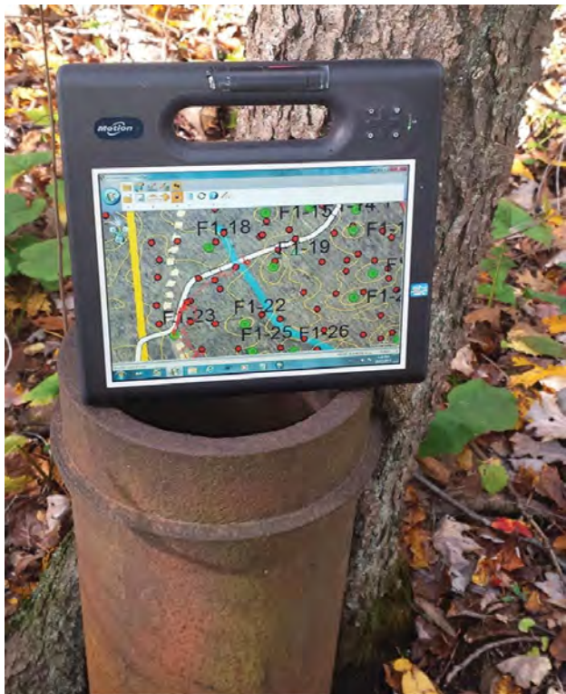
GPS-enabled computers assist researchers on the ground in finding and geolocating abandoned wells, such as the one pictured here. Source: NETL.
