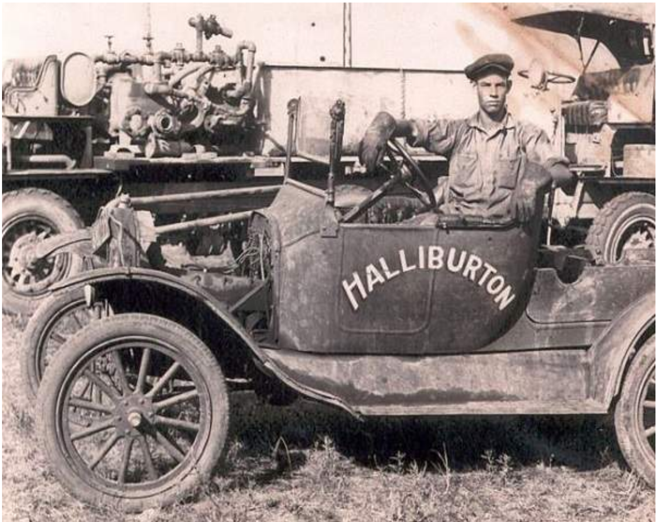
An unidentified Halliburton company employee in this circa 1920s photograph posed confidently in a Model T Ford. Background includes an early Halliburton self-propelled truck with pumps for cementing wells. Photo courtesy Timothy Johnson.
