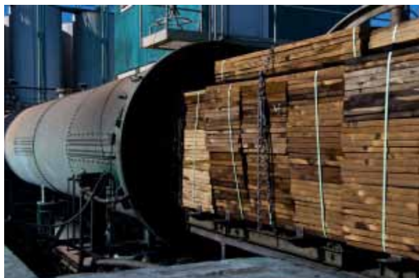
New tech: Lumber used in the construction industry enters a vessel to be pressure treated with fire retardant. The lumber then goes to a kiln where waste heat from the natural-gas-fueled engine is used to dry the wood.
