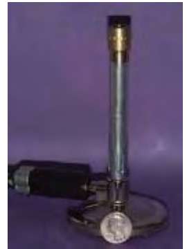
A Typical Bunsen Burner Source: DOE
